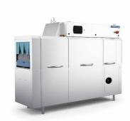
Feeding direction left-right, length 2255mm incl. Loading hood 170mm, Prewash 600mm, Chemical wash 900mm, Triple final rinse 585mm.
