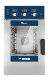
The double-glazed, left-handed door is equipped with heat-reflecting slotted glasses that, together with the air gap between the glasses, reduce heat radiation while retaining heat inside the unit, avoiding unnecessary energy loss.
