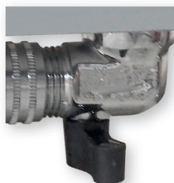
1. Control valve of steam jacket
